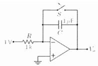
vi. In the circuit shown in the figure, the input is a 4V peak, 1 kHz square wave. 1M What is the peak-to-peak amplitude of the output waveform?
