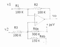
$v_o$  when  $v_1$  = 3V  $v_2$  = -2V. Consider the feedback resistance to be 100K $\Omega$
